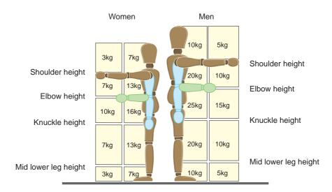
Figure 2 Lifting and lowering
