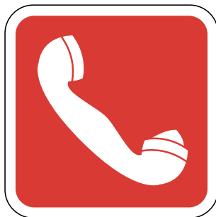
Emergency fire telephone
