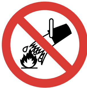
Do not extinguish with water
