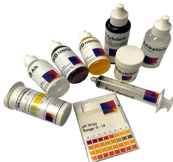
Typical Test Reagents for Site Waterside Testing and Control
