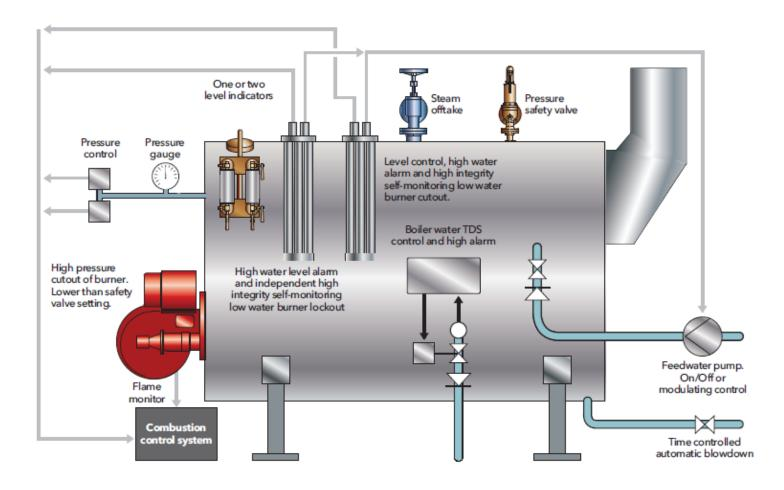
Note – for a TDS alarm to be effective, the probe must be directly mounted on the boiler shell, and not located in the blowdown line.
