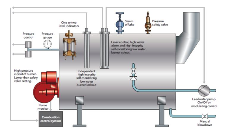
Typical equipment for the boiler:
