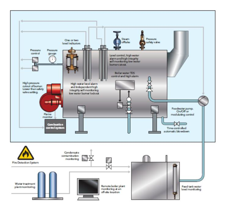
Typical additional equipment in the boiler house - 72 hours unattended is only possible with the following additional controls:
